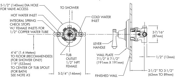
NOTE: 1. All dimensions are in inches (millimeters) unless otherwise specified and are subject to change without notice. 2. Unless otherwise specified, all inlets and outlets are ½" female copper sweat. 3. For ADA mounting locations, consult ADAAG, ANSI A117.1, or static regulations
