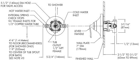
NOTE: 1. All dimensions are in inches (millimeters) unless otherwise specified and are subject to change without notice. 2. Unless otherwise specified, all inlets and outlets are ½" female copper
