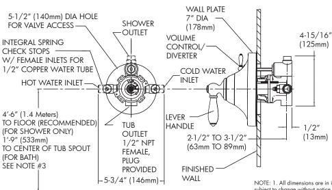
NOTE: 1. All dimensions are in inches (millimeters) unless otherwise specified and are subject to change without notice. 2. Unless otherwise specified, all inlets and outlets are  $\frac{1}{2}$ " female copper sweat. 3. For ADA mounting locations, consult ADAAG, ANSI A117.1, or static regulations
