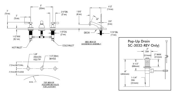
NOTE: All dimensions are in inches (millimeters) unless otherwise specified and are subject to change without notice. Lavatory inlets are sized for either coupling or sweat connections. Unless otherwise specified, all inlets are 1/2" NPSM.
