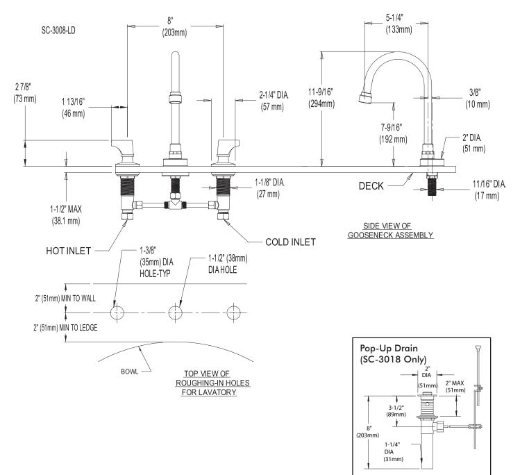
NOTE: All dimensions are in inches (millimeters) unless otherwise specified and are subject to change without notice. Lavatory inlets are sized for either coupling or sweat connections.
