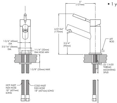
NOTE: 1. All dimensions are in inches (millimeters) unless otherwise specified and are subject to change without notice. 2. Flex hoses have 3/8 compression female threaded connections.
