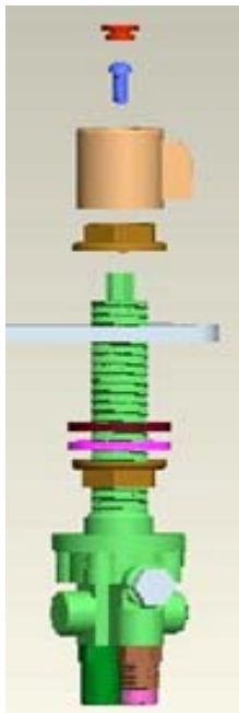
ACM (above counter mixer)
