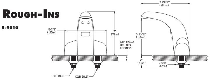
NOTE: Unless otherwise specified, all inlets are sized for either coupling or sweat connections. Unless otherwise specified, all dimensions are in inches and are subject to change without notice. Position faucet as close to the edge of the sink as possible.
