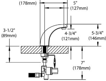
NOTE: Position faucet as close to the edge of the sink as possible. Ensure adequate clearance for wire protector, wires, washers and nut. Unless otherwise specified, all inlets are 3/8 compression with male threads. Unless otherwise specified, all dimensions are in inches and are subject to 266 change without notice.
