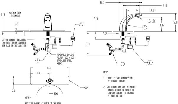
POSITION FAUCET AS CLOSE TO THE EDGE OF THE SINK AS POSSIBLE. ENSURE ADEQUATE CLEARANCE FOR WIRE PROTECTOR, WIRES, WASHERS, AND NUT.
