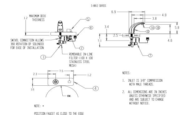
OF THE SINK AS POSSIBLE. ENSURE ADEQUATE CLEARANCE FOR WIRE PROTECTOR, WIRES,
