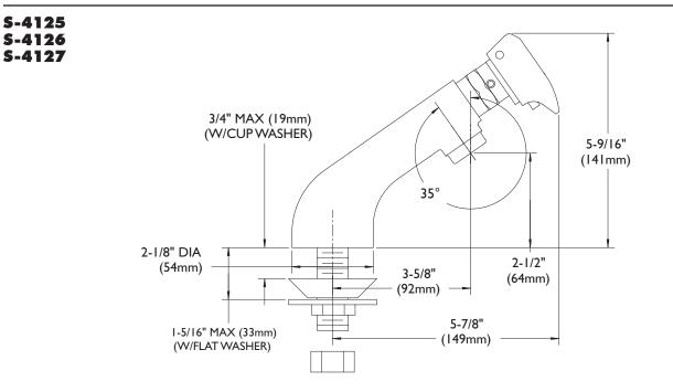
NOTE: All dimensions are in inches (millimeters) unless otherwise specified and are subject to change without notice. Inlet is sized for either coupling or sweat connections. Unless otherwise specified, inlet is 1/2" NPSM.
