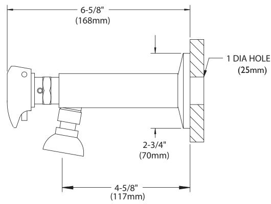
NOTE: All dimensions are in inches (millimeters) unless otherwise specified and are subject to change without notice. Inlet is 1/2" NPTF.
