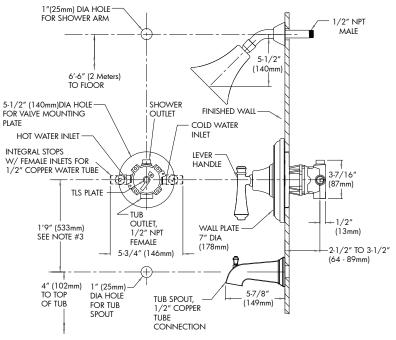
NOTE: 1. All dimensions are in inches (millimeters) unless otherwise specified and are subject to change without notice. 2. Unless otherwise specified, all inlets and outlets are  $\frac{1}{2}$ " female copper sweat. 3. For ADA mounting locations, consult ADAAG, ANSI A117.1, or
