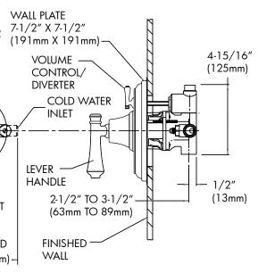
NOTE: 1. All dimensions are in inches (millimeters) unless otherwise specified and are subject to change without notice. 2. Unless otherwise specified, all inlets and outlets are  $\frac{1}{2}$ " female copper sweat. 3. For ADA mounting locations, consult ADAAG, ANSI A117.1, or static regulations
