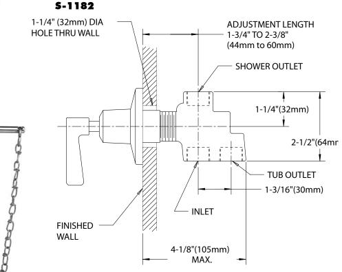
NOTE: All dimensions are in inches (millimeters) unless otherwise specified and are subject to change without notice. Inlet and outlets are 1/2'' NPT female.
